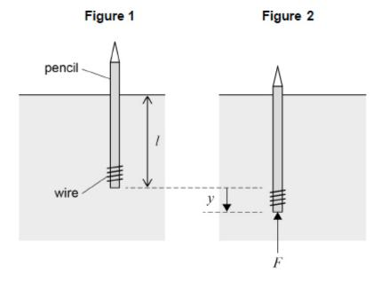
In **Figure 1** the combined weight of the pencil and wire is equal to an upwards force called the buoyancy force. The length of the pencil that is submerged is l. A student pushes the pencil down through a displacement y as shown in **Figure 2**.
