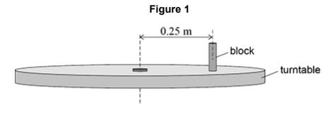
The turntable rotates with an angular speed of  $1.8\ rad\ s^{\scriptscriptstyle -1}$  and the block does not slip.
